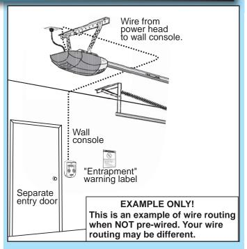
FIG.3-1 Wall Console wire routing
